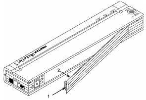
FIGURE 10. Opening the Battery Cover
